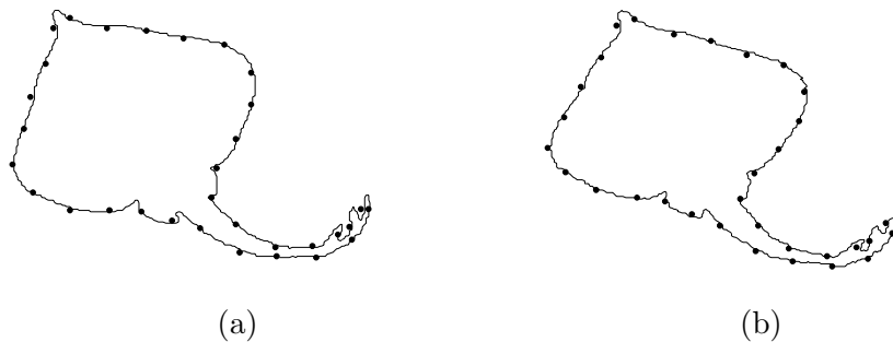
Figure 4: Points obtained by computing the Inverse DFT using only the first M = 32 Fourier coefficients for ray images: (a) Original image; (b) rotated image. The original image is super-imposed to show differences.
